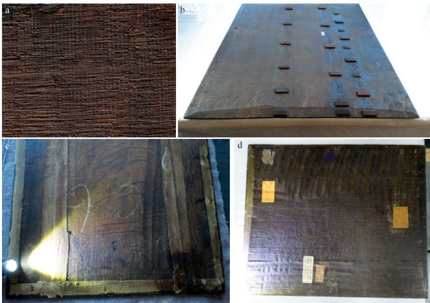
FIGURE 3 Woodworking marks observed on the panels. (a) Evenly spaced saw marks produced by mechanical sawing (this image corresponds to painting no. 16 in Table 1); (b) smooth beveled edges (painting no. 17); (c and d) local thinning by a scrub plane is found in several panels (corresponding to paintings no. 18 and 10 respectively)
